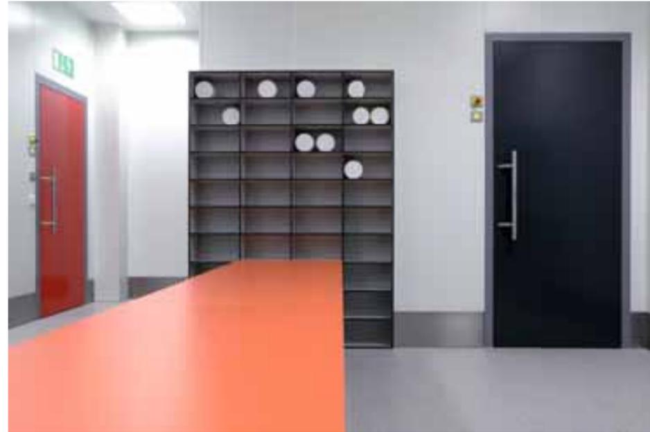
In the hameln pharma sterile production plant differentiation is generally made between four cleanroom classes in which certain particle counts are permitted and consequently appropriate gowning procedures are required. The personnel lock system that links all the different cleanroom classes together is designed to allow for standardized procedures.
